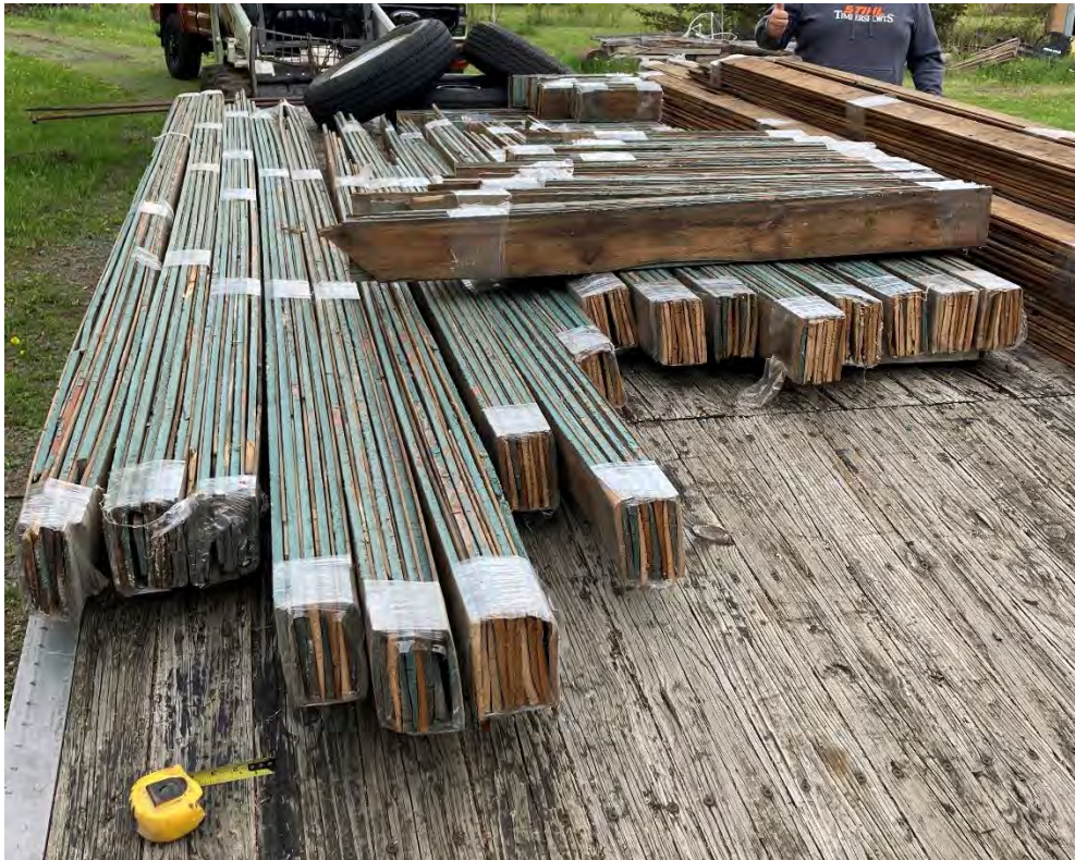
Figure 9 – Clapboard siding and interior sheathing boards on trailer.
