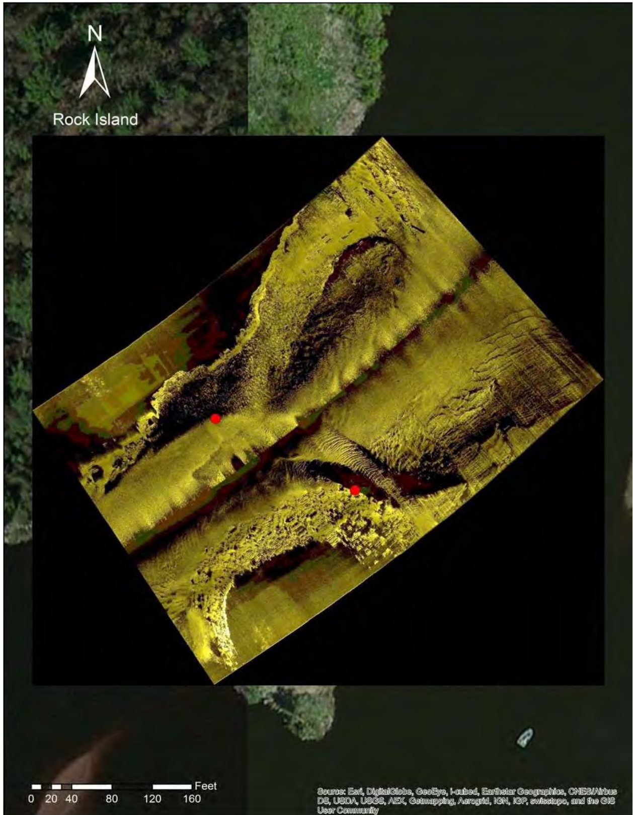
FIGURE 29. Sonar imagery around Rock Island identified as natural rock outcroppings.
