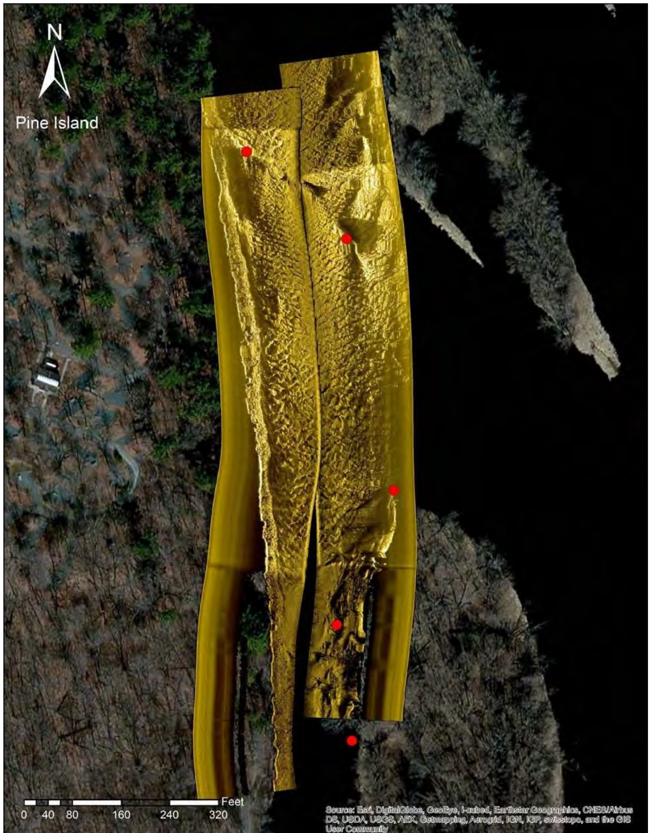
FIGURE 102. The sonar imagery from upper Pine Island showing the large wing dam labeled PinelandsLargeWingDam.
