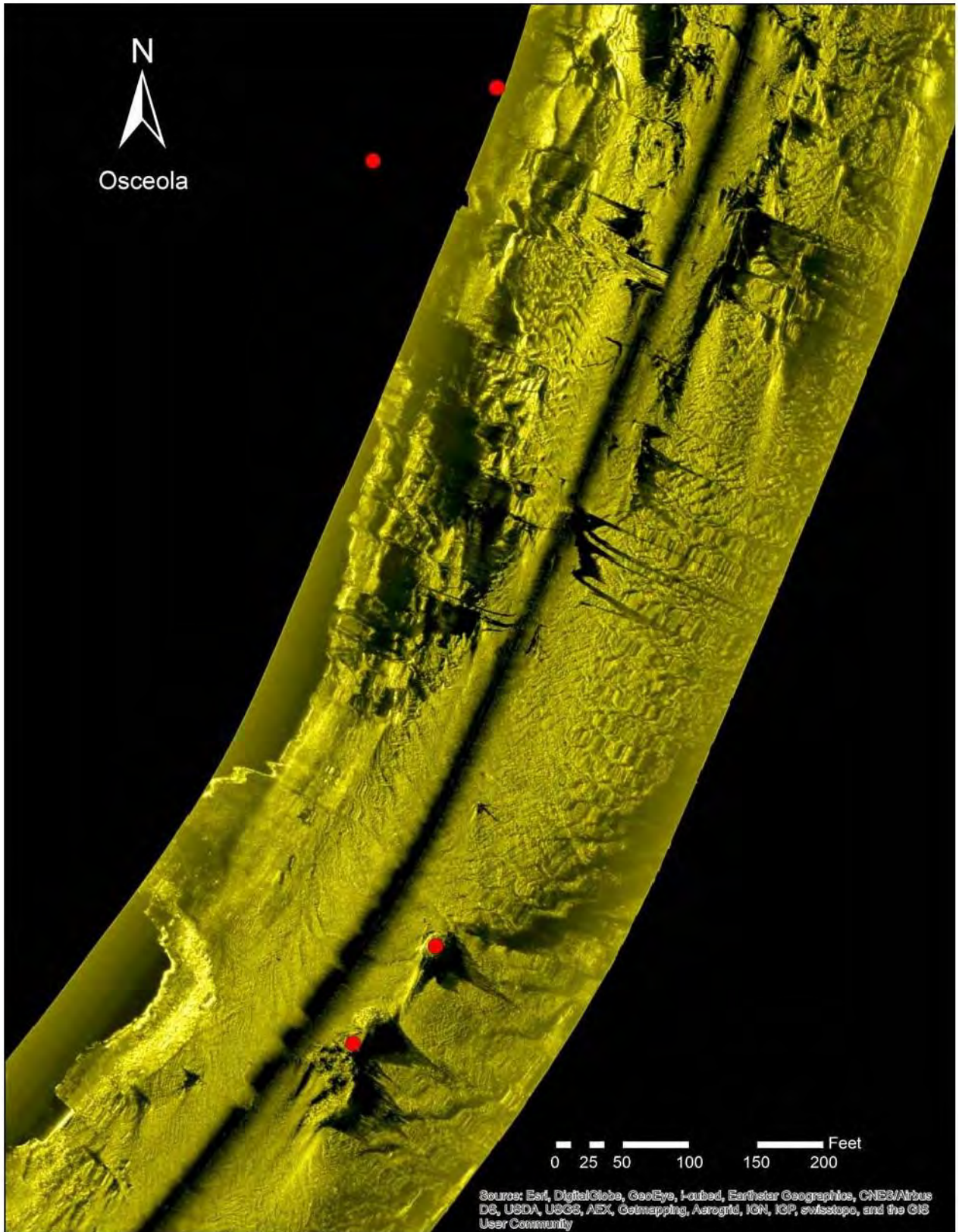
FIGURE 61. Sonar imagery from Osceola showing two structures possibly associated with construction of the previous bridge.
