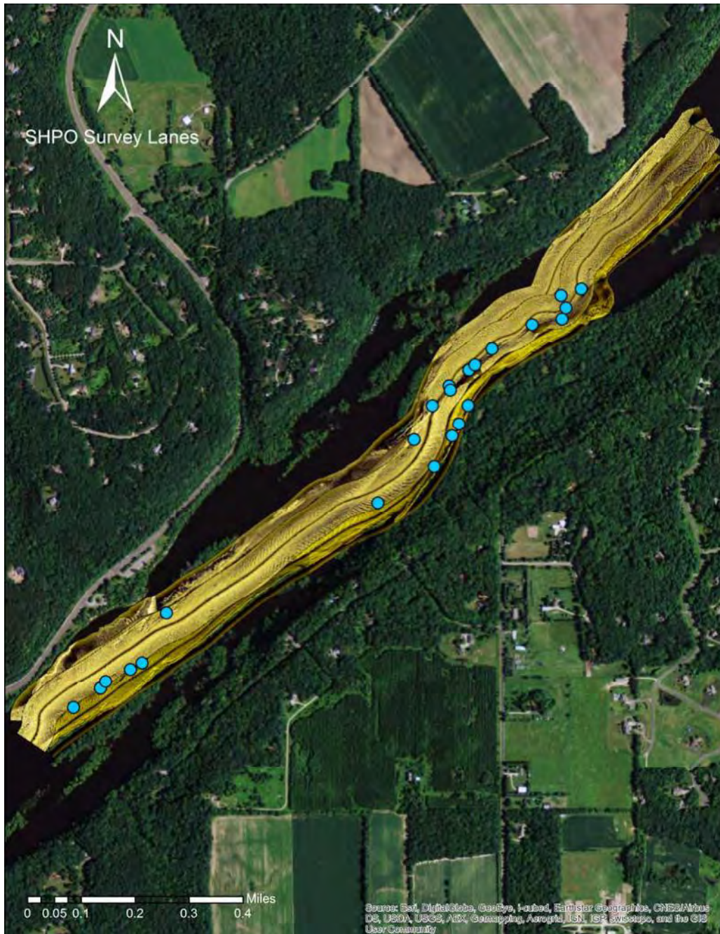
FIGURE 152. ESRI aerial map with the Stillwater Boom Ground sonar survey and identified targets.
