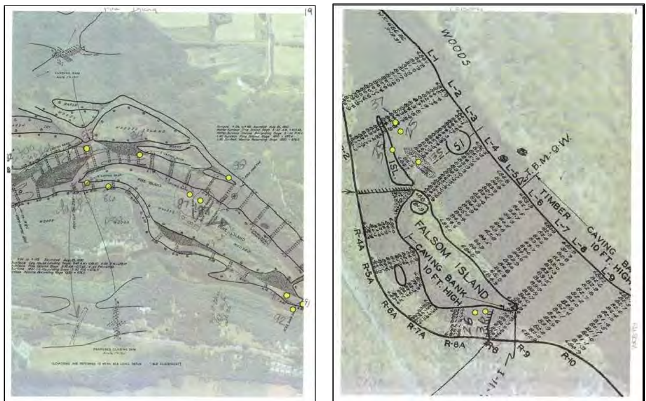
FIGURES 1 and 2. GIS maps of Folsom and Boom Islands with layers of GPS targets (yellow dots) and the rectified 1937 USACE map.
